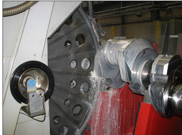
Fig. 2. The Molemab B126-100639 S.630090 grinding wheel during the operation
