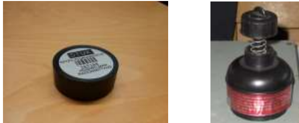
Figure 7. Radon samplers used in Finland (on the left) and in Lithuania.
