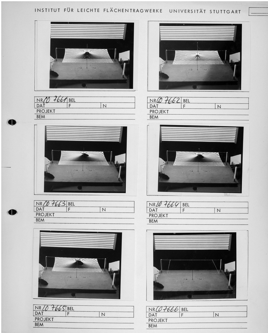
Ill. 7 : Maquettes en bulles de savon, Institute for Lightweight Structures (IL) de l'Université de Stuttgart, planche contact, vers 1965. © saai / Archive for Architecture and Civil Engineering, Karlsruhe Institute for Technology.
