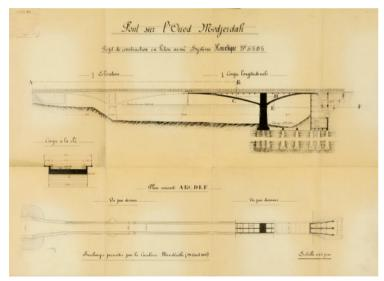
competitive bidding was opened instead, Hennebique's engineers preferred to submit a cantilever bridge (with a central span of 56 m). This change required the use of Compressol for the pilings and therefore the services of the Hennebique subsidiary Fondations par Compression Mécanique du Sol. The latter company finally obtained the contract in its entirety after the withdrawal of the initial
