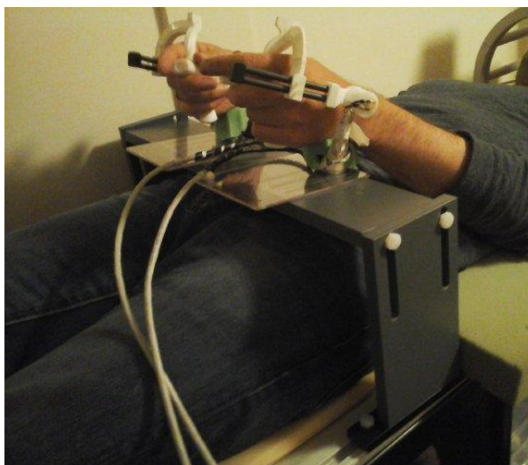
Figure 3.8: Device in use: resting position adopted by the participants. This particular example corresponds to the training setting. Anatomical variability is covered by hardware adaptations discussed in Section 3.1.
