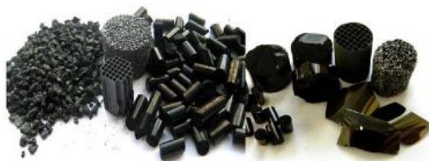
Figure 3.10- Carbon materials obtained in different morphologies: grains, powders, pellets, films and coatings on monolith and foam structures (Morales-Torres, Carrasco-Marín, et al. , 2015).
