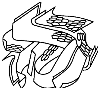
Figure 3.6- Schematic representation of the microstructure of activated carbons (Bansal, Donnet, et al., 1988).
