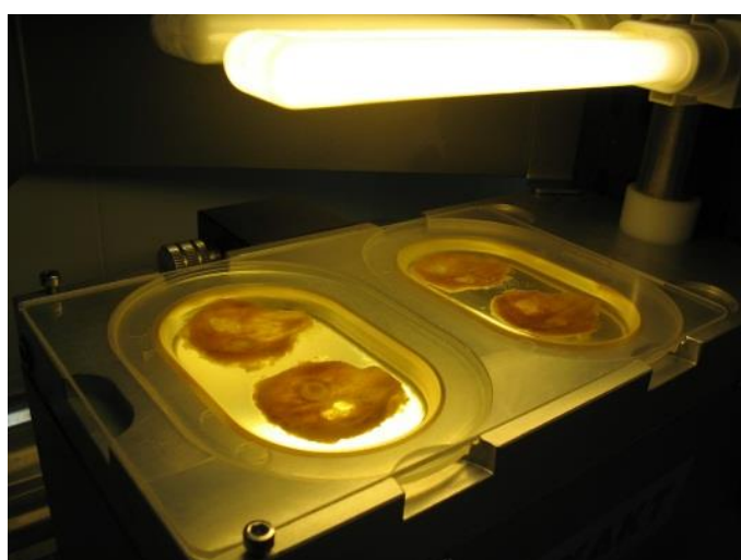
Figure 2.35. Exakt 520 Light Polymerization Unit (Exakt, Hamburg, Germany) during the yellow light cycle.
