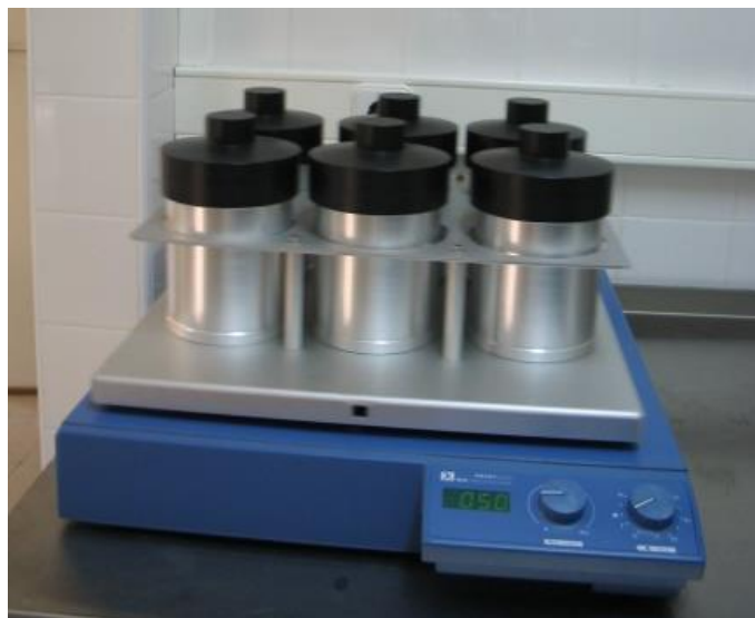
Figure 2.34. Dehydration and infiltration unit (Jkika Labortechnik HS 501 digital ® , Exakt-dehydration and infiltration unit, Exakt, Hamburg, Germany).
