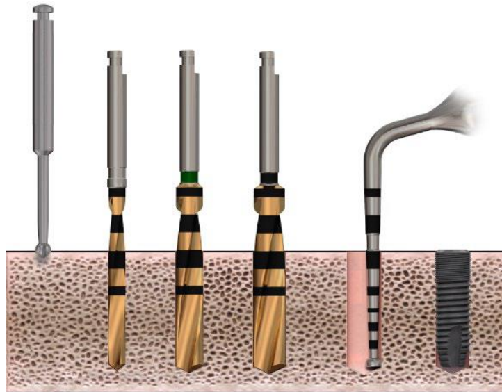
Figure 2.16. Drilling sequence for the titanium implants (Taken from Astra Tech ® Product Catalog).
