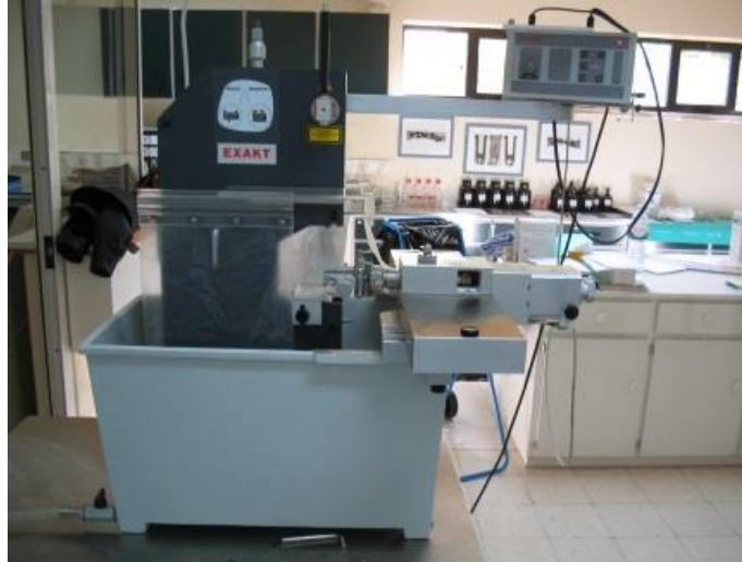
Figure 2.37. Hard tissue microtome for dividing the block into two equal sections (Exakt® 300 CP Precision Parallel Control, Exakt®, Hamburg, Germany).
