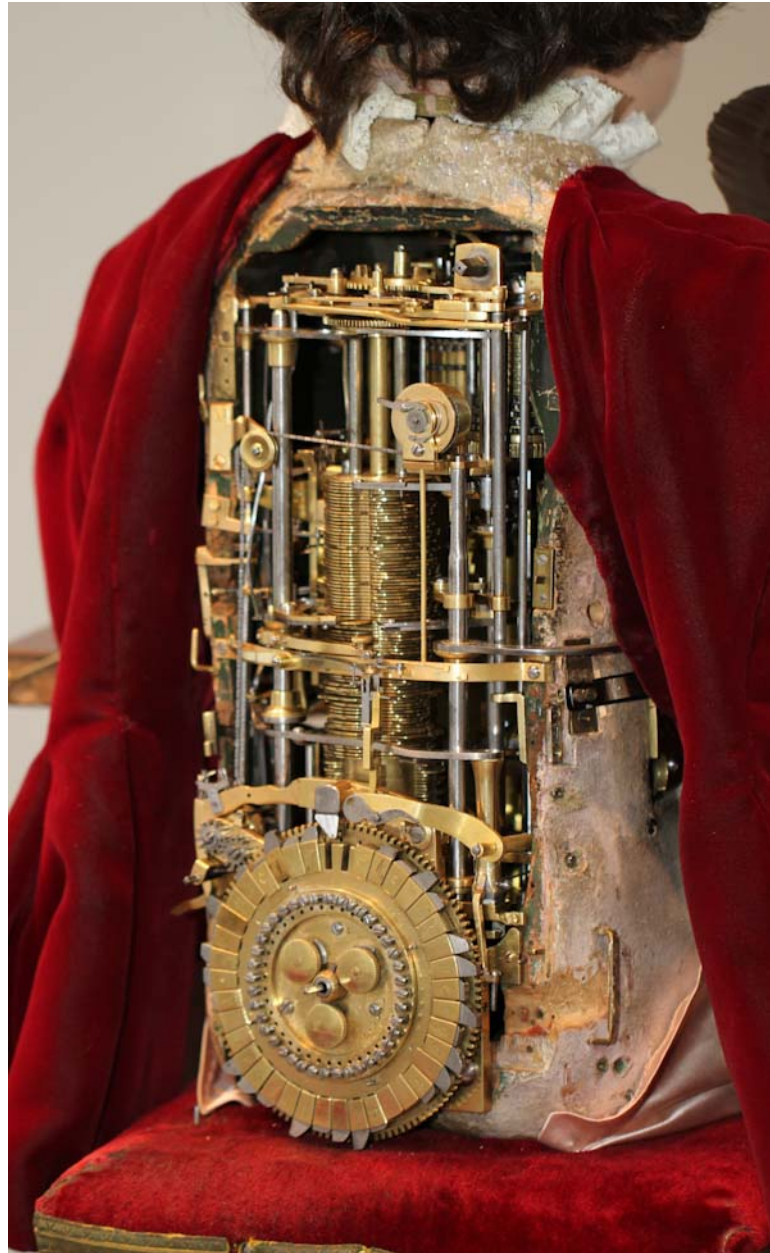
Figure 2.3: A view of the rear of L'Ecrivain, showing the mechanism and the configuration wheel holding 38 of 40 tabs. Used with permission of Ariel Adams, from http://www.ablogtowatch.com/jaquet-droz-the-writer-automata-awesome-antique-android/
