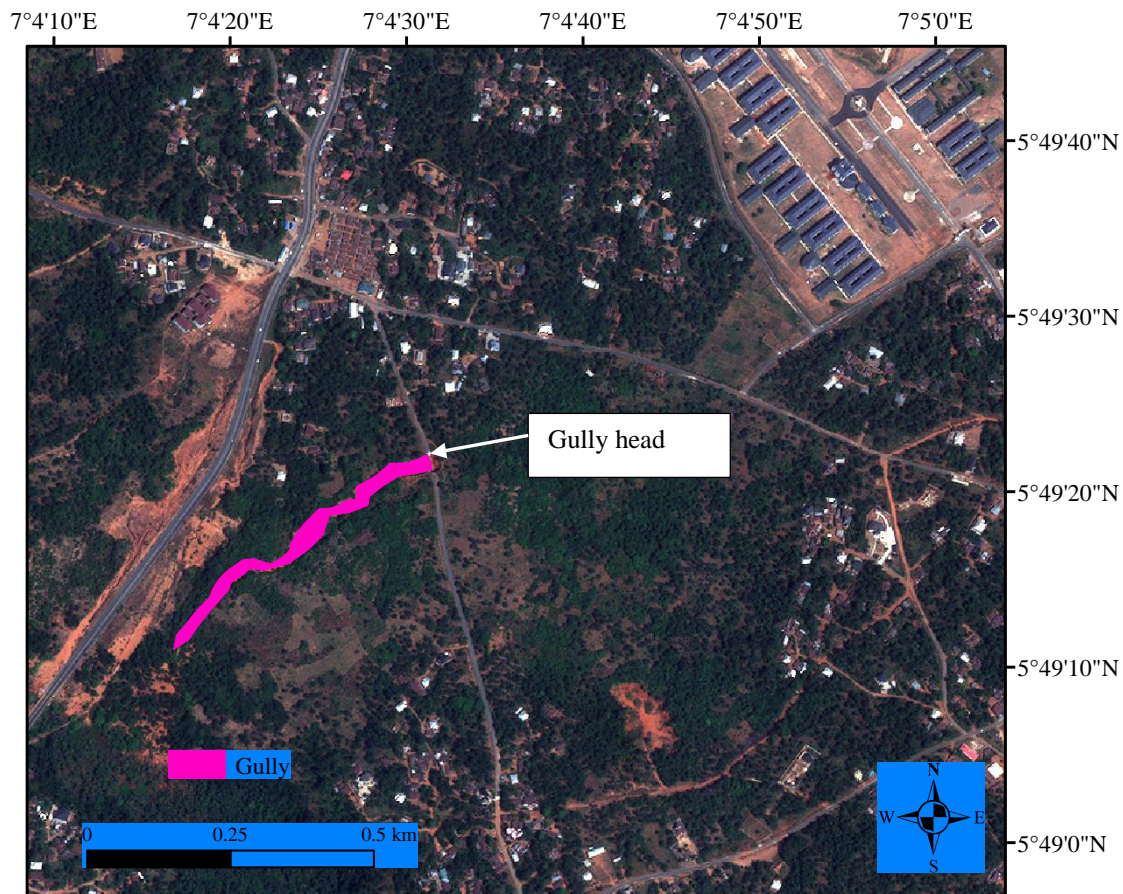
Figure 4.23: 2017 satellite data showing IdeatoSouth_gully2. The gully was first identified in the 2014 satellite data but in 2017, it had destroyed one of the tarmac roads as shown in the satellite data.
