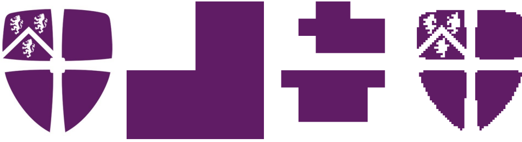
Figure 2.2: An example of a possible material parameter within a cell (left). A three stage splitting of the cell into regular grids of subcells, to capture the material data with increasing accuracy. The subcells have resolutions of 2 \times 2 , 8 \times 8 , and 64 \times 64 (right).
