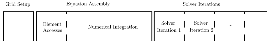
Figure 6.3: Conventional sequential matrix equation assembly. The mesh is assembled and then exact numerical integration of equations is performed before the solver iterations begin.
