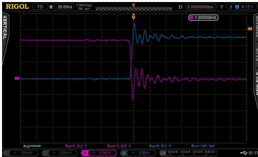
Figure 50: Measured Turn ON (OFF) Characteristics of Upper (Lower) Transistors
