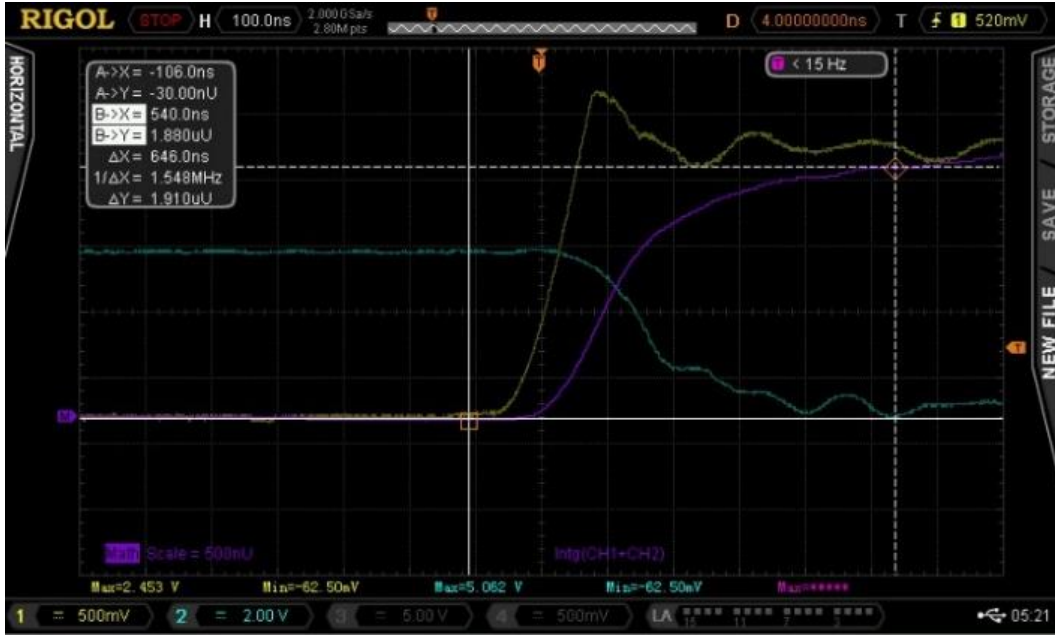
Figure 34: 8 Amp, Switching OFF waveform with calculations
