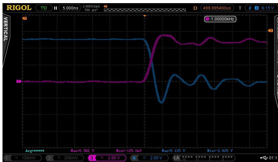
Figure 51: Measured Turn OFF (ON) Characteristic of Upper (Lower) Transistors
