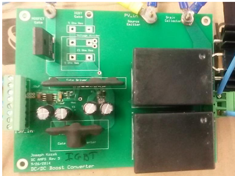
Figure 18: Populated DC/DC Boost Converter Gate PCB
