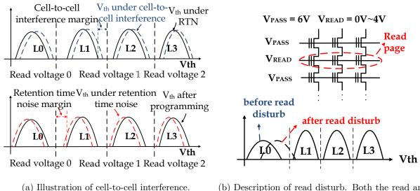
(b) Description of read disturb. Both the read and unread cells are exposed to risk of read disturb.
