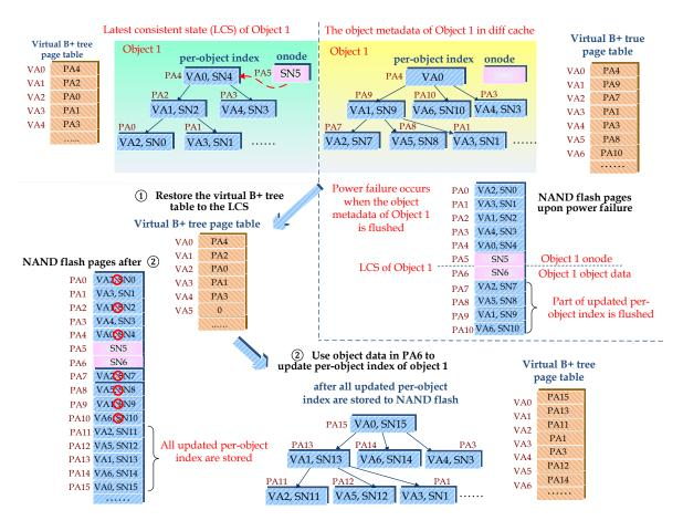
Figure 33: An example of per-object index recovery.
