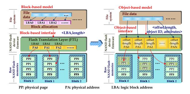
Figure 1: The block-based storage v.s. the object-based storage.
