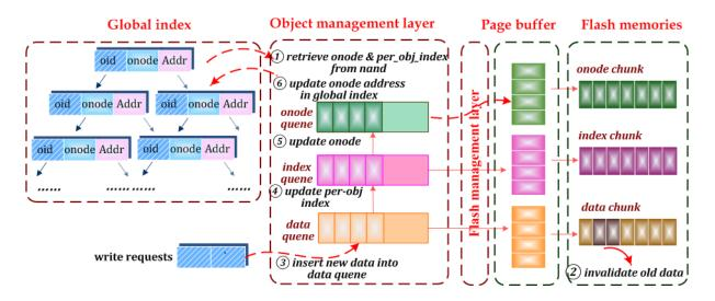
Figure 38: The ObjNandSim write I/O flows.
