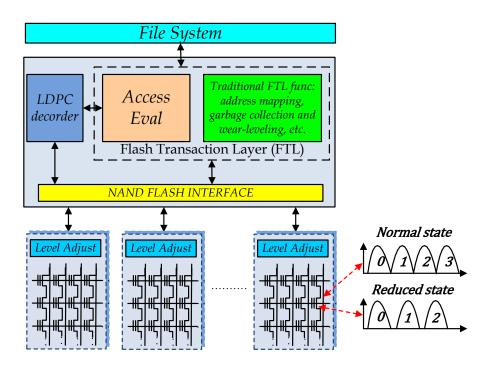
Figure 16: FlexLevel NAND flash storage system overview
