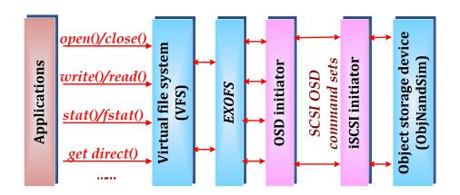
Figure 35: The architecture of simulation platform.
