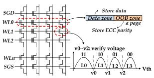
(b) MLC NAND flash device structure and the  $V_{th}$  distribution.
