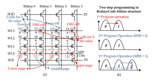
Figure 17: ReduceCode bitline structure.
