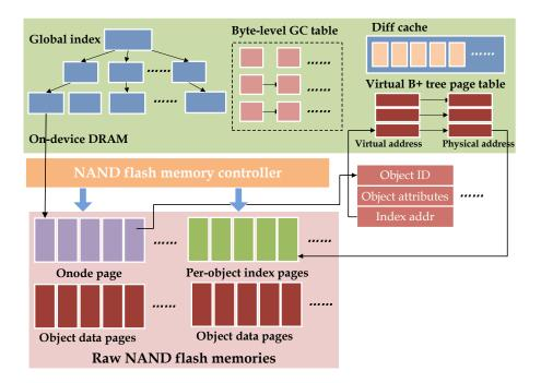
Figure 28: The overall architecture of the DMM device.
