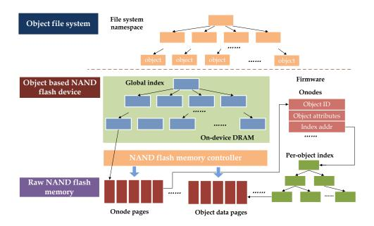
Figure 26: The architecture of object-based storage system.
