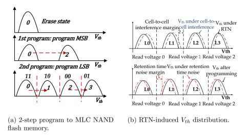
Figure 3: The program method and RTN noise of NAND flash memory.
