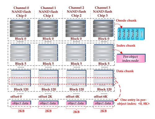
Figure 46: The data layout of existing ONFD.
