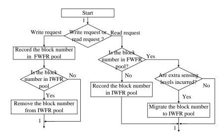
Figure 21: IWFR identification flow.
