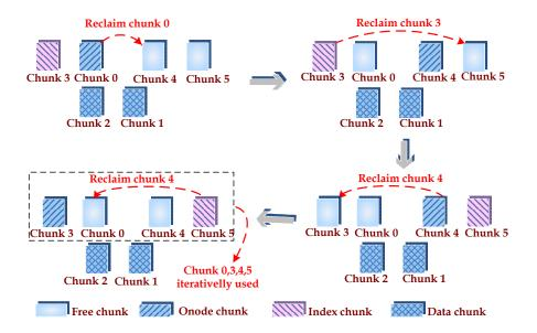
Figure 47: The biased chunk reclamation issue in ONFD.
