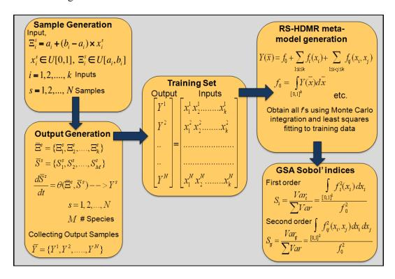
Figure 2.2 Workflow for the entire global sensitivity analysis using RS-HDMR.
