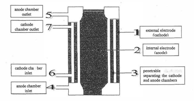
Figure 1.1: Flow-through Electrochemical Modular, FEM<sup>13</sup>
