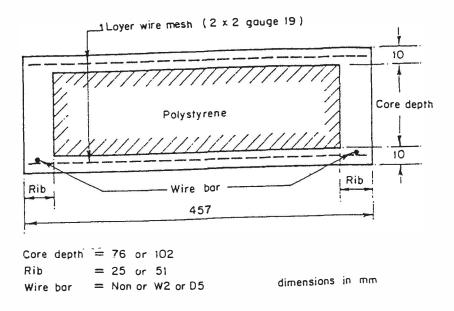
Figure 1: Typical Bending Specimen Cross-section
