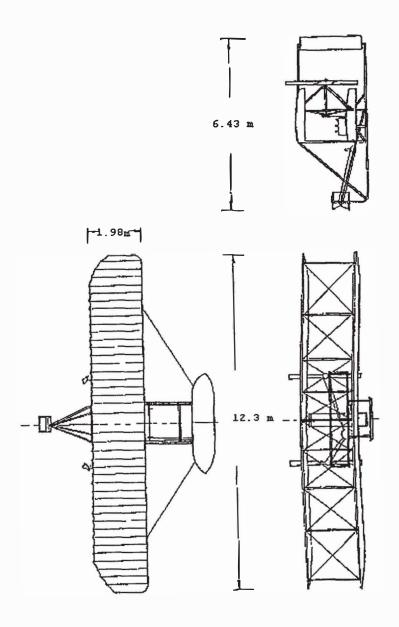
Figure 3: Views of the First Airplane Used by Wright Brothers in 1903 (McCormick, 1995).
