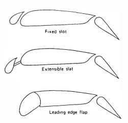
Figure 1: Some Multi-Component Airfoil Configurations (McCormick, 1995).
