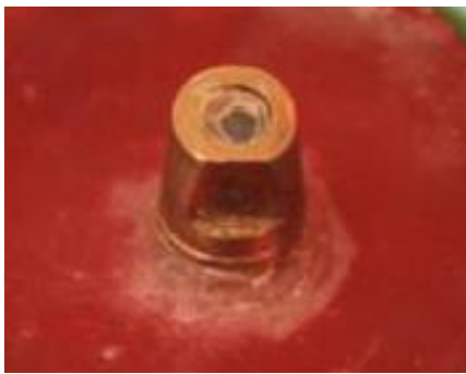
Figure 1: Brass die embedded in acrylic resin block
