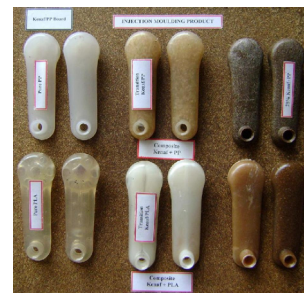
Figure 1: Examples of car door handles from kenaf fibre
