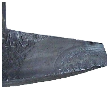
Figure 2. Transverse defect (foot fracture)
