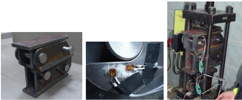
a) installation of tenseters on the model of the kvik-capler
