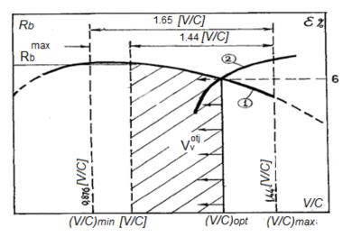
1 is the curve of changes in the strength of concrete; 2 is the compression curve of the cement paste.
