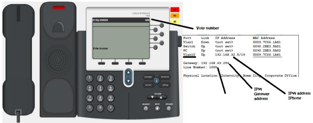
Figure 9. Output of a configured Cisco IP phone ready to make calls over Ipv4/IPv6 (Researcher, 2020)
