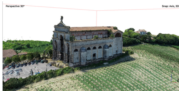
Figure 4: Final point cloud.
