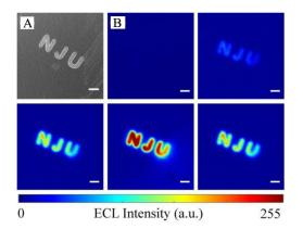
**Figure 3** (A) SEM image of the "NJU" pattern created by photoresist on one side of the array. (B) Five ECL snapshots recorded from a potential sweep experiment for detection of 100  $\mu$ mol·L<sup>-1</sup> Fe(CN)<sub>6</sub><sup>3-</sup> in the cathodic pole using 1 mmol·L<sup>-1</sup> Ru(bpy)<sub>3</sub><sup>2+</sup>, 50 mmol·L<sup>-1</sup> TPrA and 100 mmol·L<sup>-1</sup> phosphate buffer (pH = 7.5) in the presence of 0.05% FSN in the anodic pole. Scale bars are 20  $\mu$ m.
