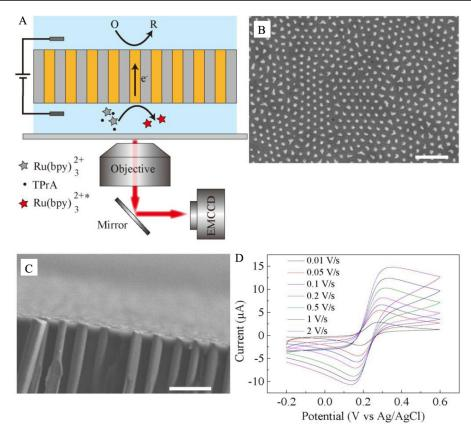
**Figure 1** (A) Schematic illustrating the principle of electrochemical imaging. (B) Top view SEM image of the nanoelectrode array with 200 nm diameter and 450 nm pitch. The scale bar is 2  $\mu$ m. (C) Cross-section SEM image of the nanoelectrode array. The scale bar is 1  $\mu$ m. (D) Voltammetric responses of the array at different scan rates. The electrolyte contained 1 mmol·L<sup>-1</sup> K<sub>4</sub>Fe(CN)<sub>6</sub> and 0.1 mol·L<sup>-1</sup> NaCl. (color on line)
