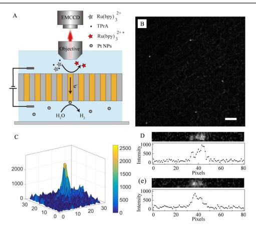
**Figure 5** (A) Schematic of ECL imaging on single bipolar nanoelectrodes. (B) A representative ECL image of single bipolar nanoelectrodes. The scale bar is 20  $\mu$ m. (C) A typical 32×32 pixels 3D ECL intensity surface plot of a single nanoelectrode. (D, E) ECL images of three (D) and two (E) adjacent nanoelectrodes and the corresponding intensity line profiles.
