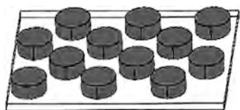
Fig. 1. Magnetic system of cylindrical permanent magnets arranged in a checkerboard pattern
