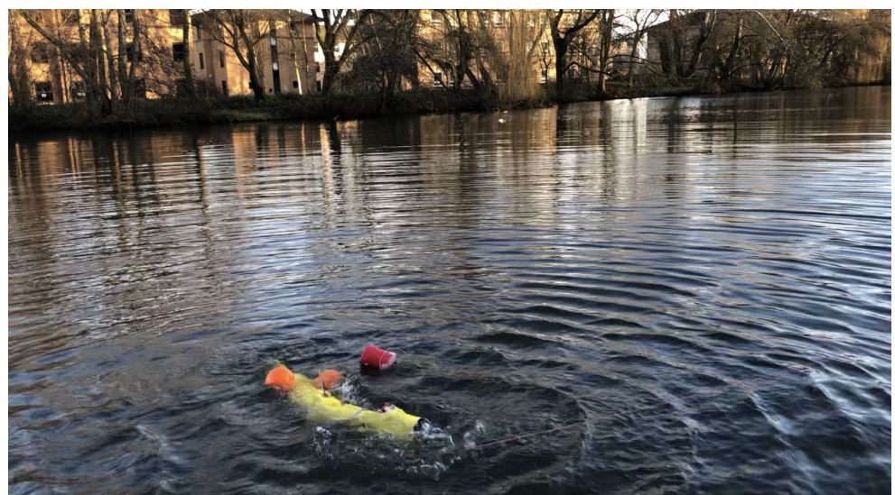
Figure 17. RoboFish prototype Swimming on the Surface of a Lake: two side plastic buoys were included to maintain positive buoyancy; a rope is attached to it to be dragged to the home point in the case of failure or battery recharge.
