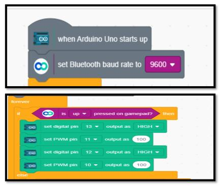
The next block describes the command that the Arduino UNO microcontroller will send to the Motor that drives the GeoBot. Referring to the diagram above, the command is a forward movement when the upward pointer game pad is pressed.
