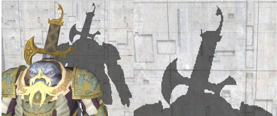
Figure 3.7.b: A basic shadow map with jagged edge aliasing artefacts
