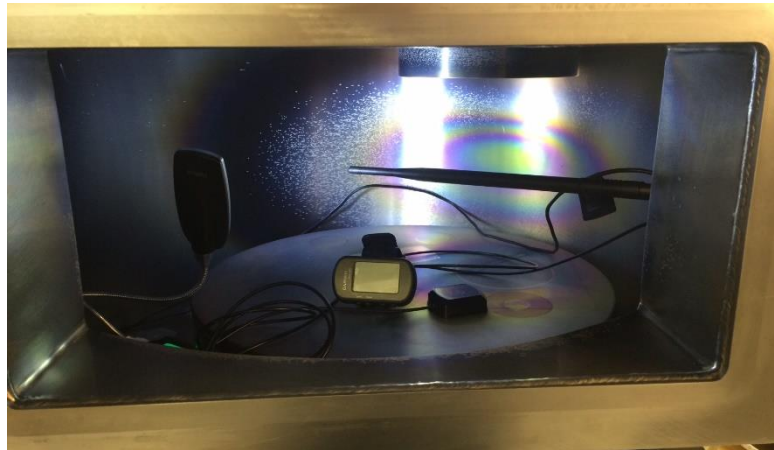
Figure 19 -RF shielded chamber with victim and spoofing antennas
