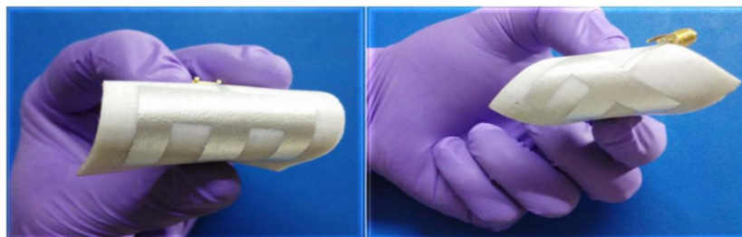
Figure 2-8 : Screen printed antenna on polyester fabric [37].
