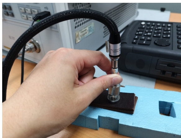
Figure 4-3 : The measurement setup for the electric properties of the leather.
