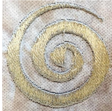
Figure 2-2 : Example planar antenna fabricated with conductive threads [21].
