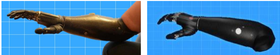
Figure 2: To the right, the real Bebionic prosthetic arm. To the left, the VR Bebionic 3D model of the prosthetic arm.
