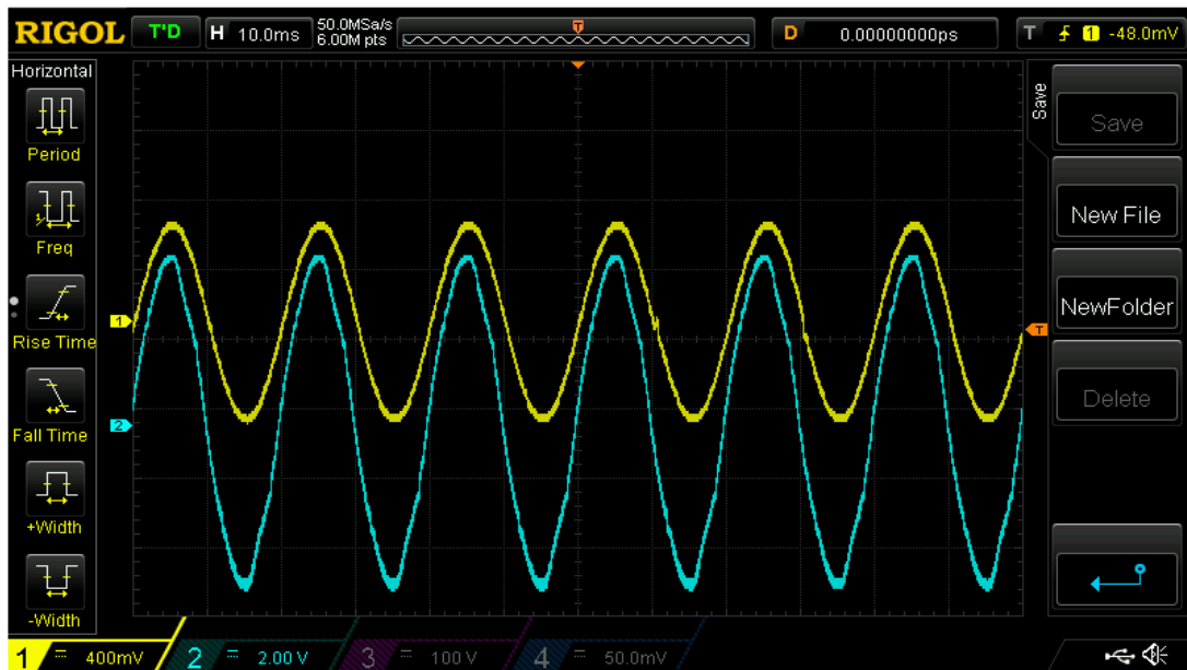
Figure 10. Waveform of Frequency and Phase Lock
