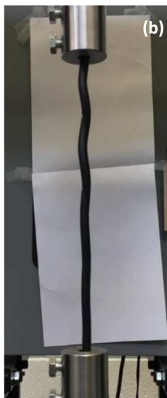
Fig. 9. (a) All three tensile tested HAYs, (b) frictional forces after the epoxy resin failed, and (c) failure of epoxy resin from experiment 3 – (A) area subjected to stress from the bolt in the chuck (B) remaining part of the nitinol wire after failure.
