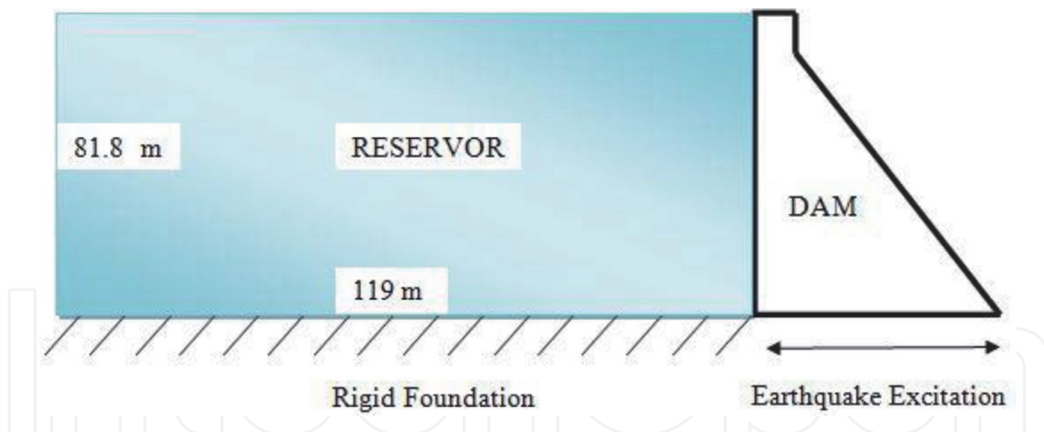
Figure 5. Dam-reservoir model used to study hydrodynamic pressure on the Kinta RCC dam.
