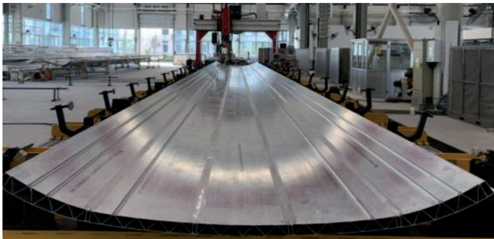
Figure 19. Laser-MIG weld machine for roof of aluminum car-body of high speed train.
