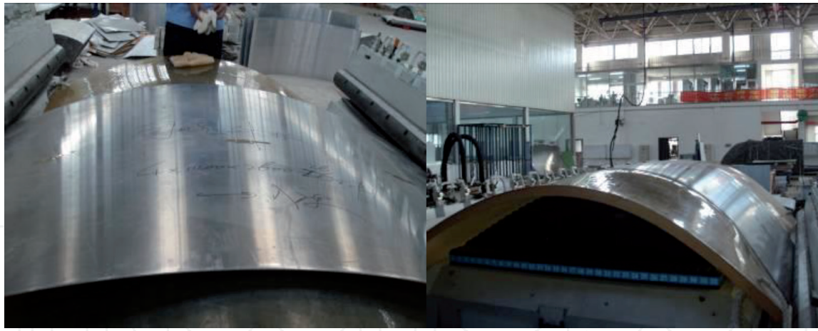
Figure 14. Skin drawing based on flexible multi-point die.
