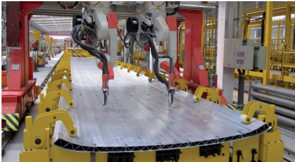
Figure 3. Typical sidewall of high speed train composed of extruded sections.
