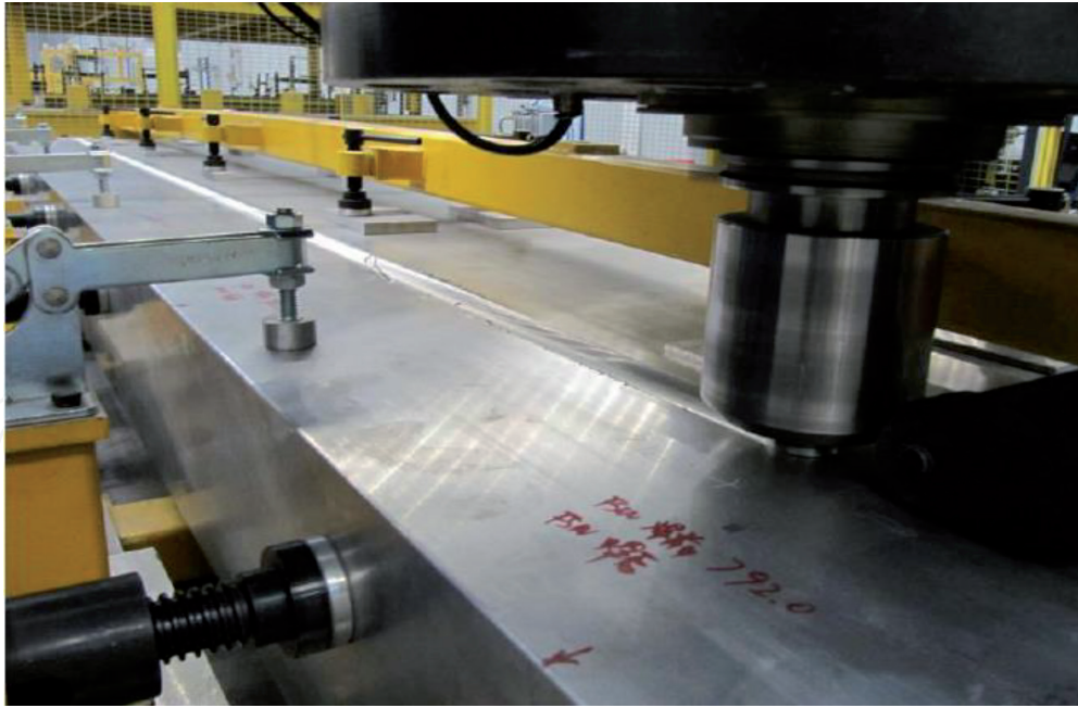
Figure 17. FSW process of a sleeper beam.
