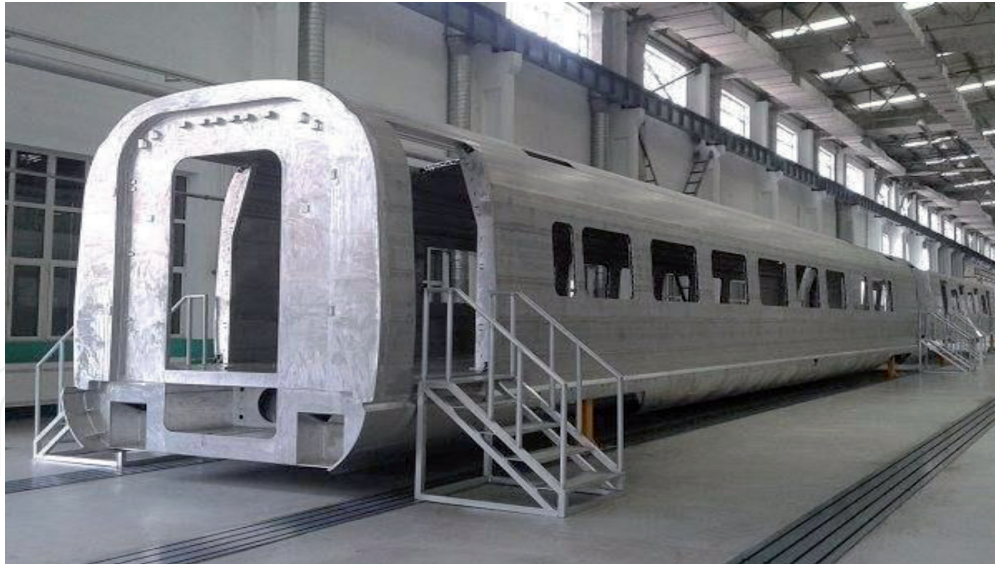
Figure 2. Typical car-body of high speed train made of aluminum alloy.
