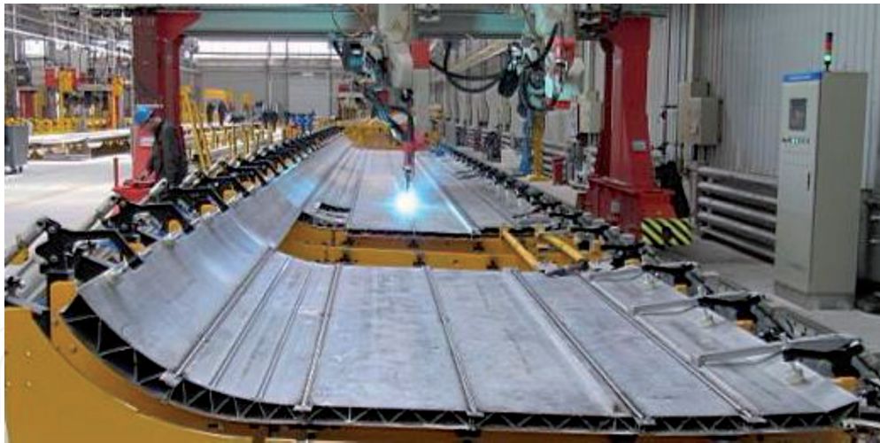
Figure 15. Automatically MIG welding process.
