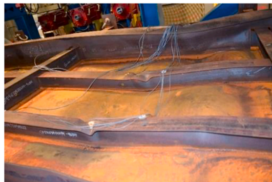
Fig. 8. View of the final deformed structure shape in Section 2 illustrating the plate buckling, stiffener buckling, and girder tripping buckling modes.
