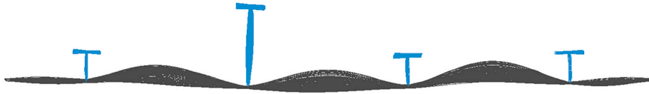
Fig. 11. Example of the measured imperfections applied to the FE model (plate and longitudinal stiffeners, values magnified by a factor of 10 for clarity).
