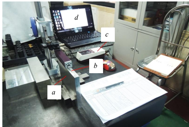
Fig. 5. Surface roughness measurement system: a – Workpiece; b – Surface roughness sensor; c – Data processing; d – PC and software
