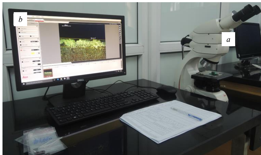
Fig. 4. Tool wear measurement system: a – Microscope; b – Processing system
