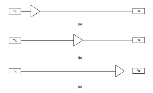
Figure 1.1: Optical fiber amplifier classification; (a) Post amplifier (b) Inline amplifier (c) Preamplifier
