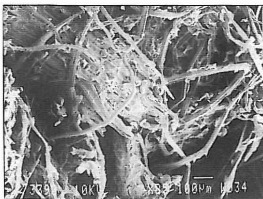
Fig 2: Wood fiber of oil palm stem after steam explosion at 25 kgf/cm 2 for 10 min. The area "A" shows a bundle of intact fibers.
