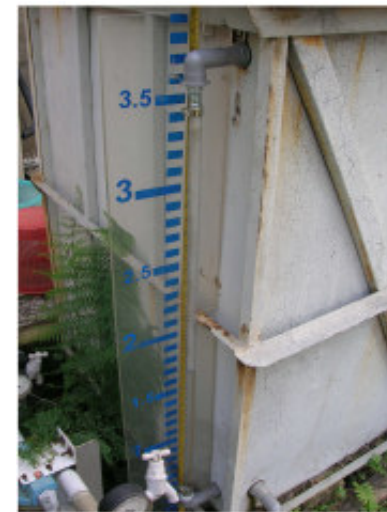
Figure 2: The scale for measuring water depth in the tank.
