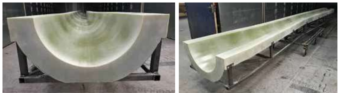
Figure 1. Blade mould half after curing.
