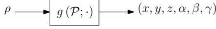
Fig. 5: Estimation mapping between the received SNR and the 3D position and the 3D orientation angles of the UE.
