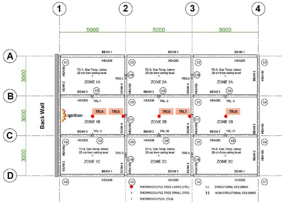
Figure 1- Layout plan of the test compartment and location of TRL4 to TRL8 (dimensions in mm)
