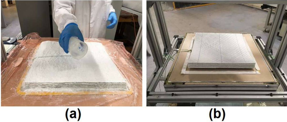
5 Figure 3. Lay-up of the thick-section laminates on the heated tool: (a) GRN 918 epoxy powder was 6 weighed and then manually dispersed between each layer of GF fabric; (b) semi-preg plies were cut and 7 stacked on the heated tool.
