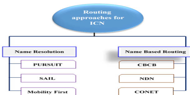
Fig 1: Routing Approaches in ICN Architectures
