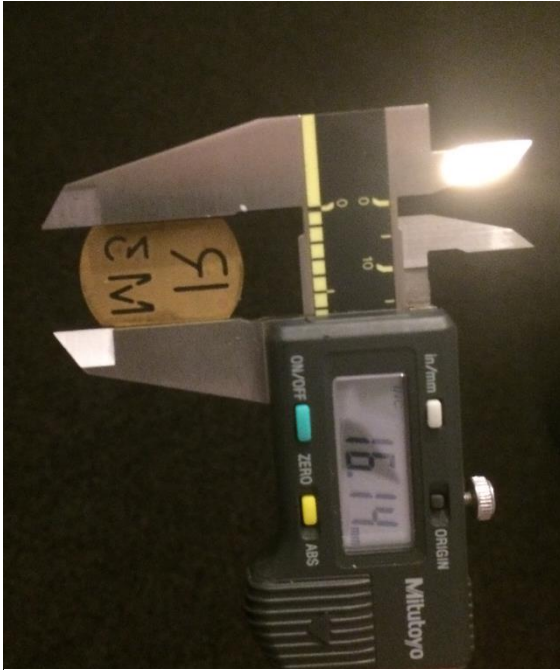
Figure 3.11. Photograph of calliper measuring the mediolateral dimensions of the marker
