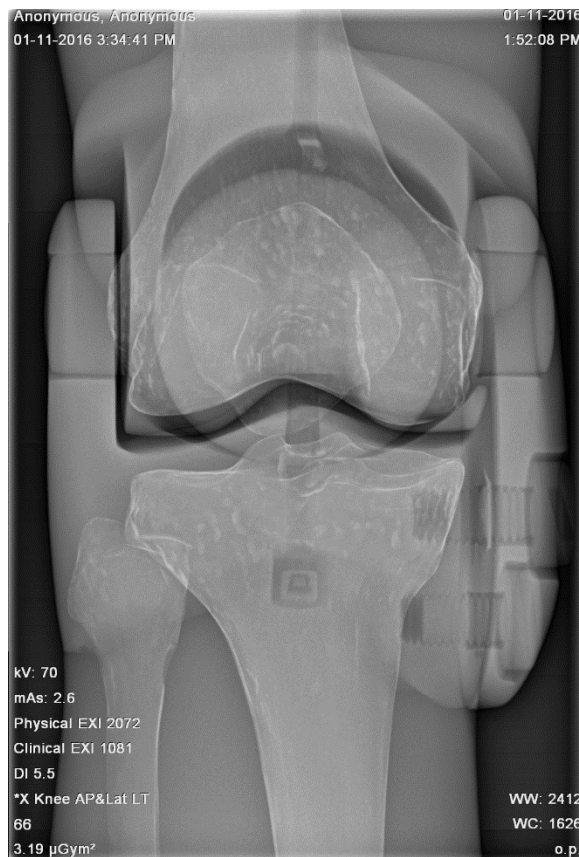
Figure 3.3. X-ray of whole body phantom (PBU-50) to determine knee length and collimation requirements
