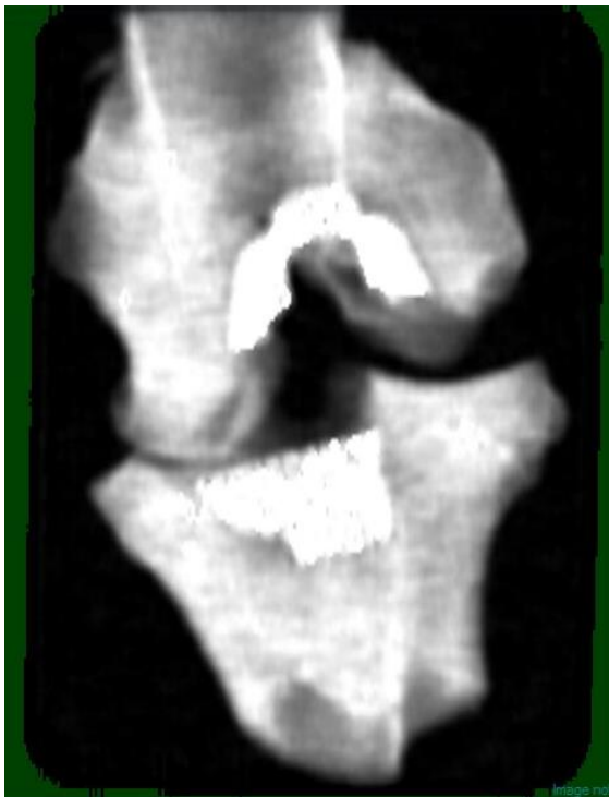
Figure 3.19. DXA scan ( thin setting ), of cones and bones in 15 cm water
