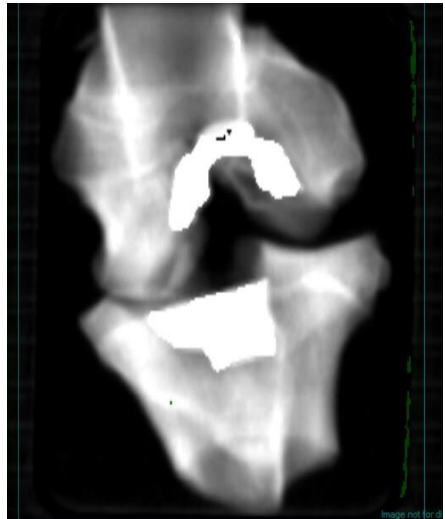
Figure 3.20. DXA scan ( standard setting ), of cones and bones in 15 cm water
