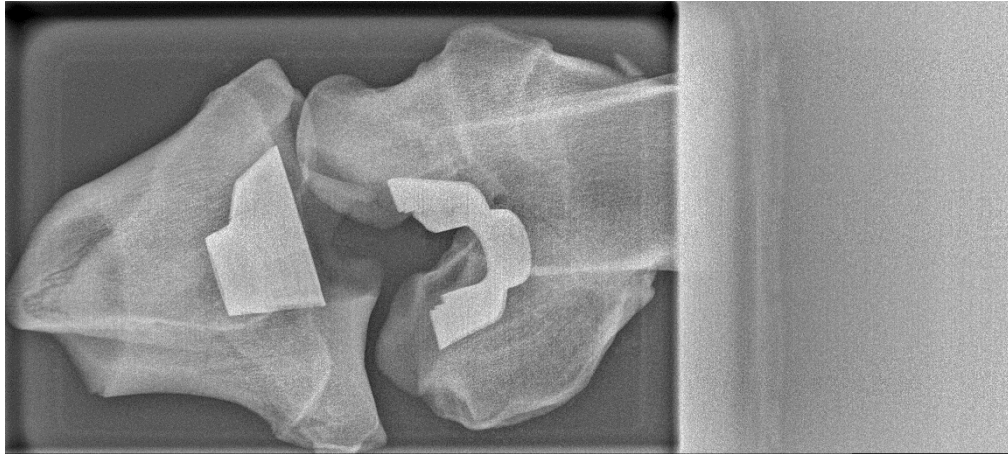
Figure 3.28. X-ray of baseline image of cow cones on exposure setting 60 kVp 2.5 mAs, showing stretched canvas issue
