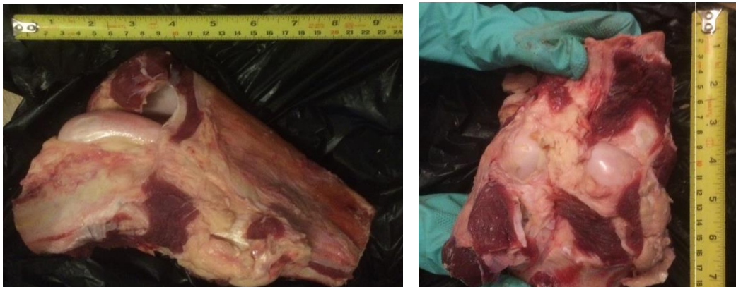
Figure 3.4. Photographs of the left bovine femur, tibia and patella, showing the amount of tendons, ligaments and muscles still on the bone that needed to be removed prior to insertion/ scanning. Measuring tape used to show size.
