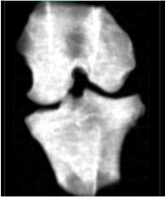
Figure 3.17. DXA scan ( thin mode ) of cow bones in 15 cm of water in plastic container
