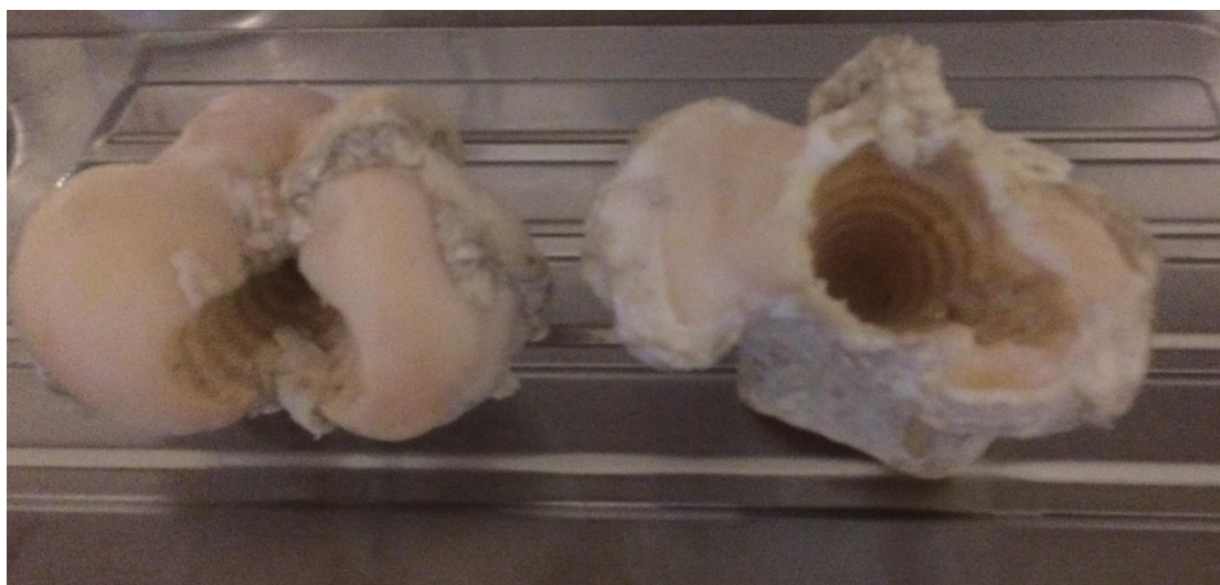
Figure 3.5. Photographs of the bovine tibia (right) and femur (left) with the cavities for the implants to be inserted created.
