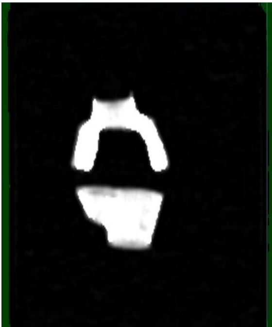
Figure 3.13. DXA scan of just the cones submerged in water (thin setting)
