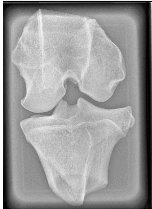
Figure 3.18. X-ray (81kv 3.2 mAs) of cow bones in 15 cm of water in plastic container
