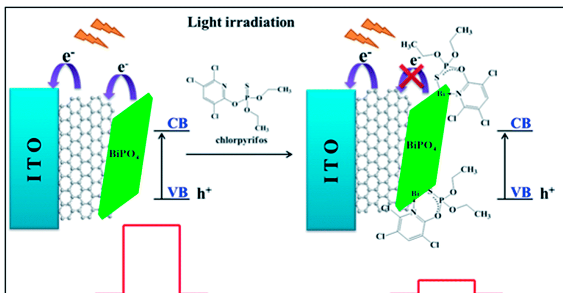
Figure 13. The PEC sensor illustration for chlorpyrifos. Adapted from ref [182].
