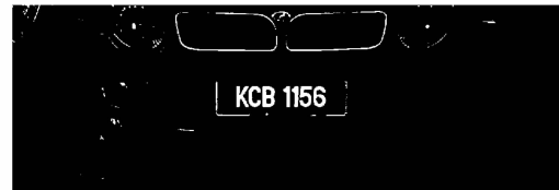
Figure 11. Image after converted to binary image
