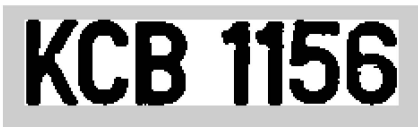
Figure 14. Image show that the car plate had been crop from the binary image
