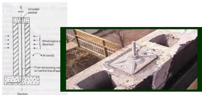
a) Post-tensioned masonry diaphragm walls
