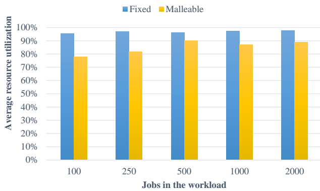
Figure 8. Average resource utilization on different fixed and malleable workloads with an increasing number of jobs.
